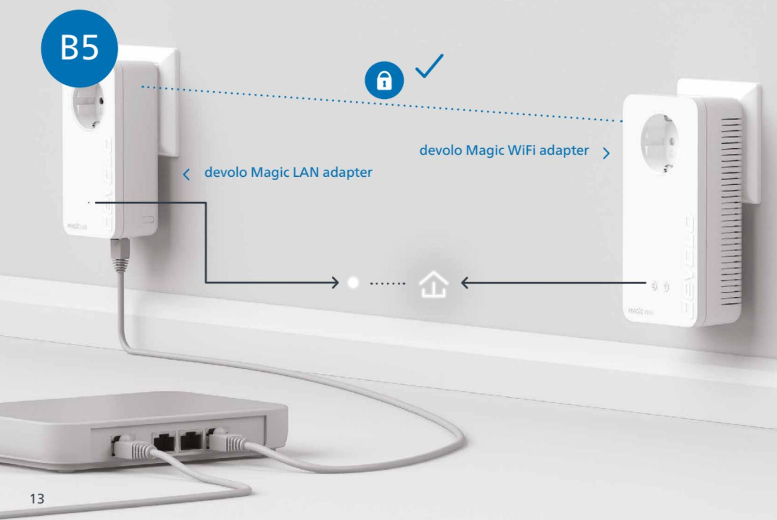
**| EN |** The process is complete as soon as all of the LEDs on the devices light up solid white. The process takes a maximum of 3 minutes.
