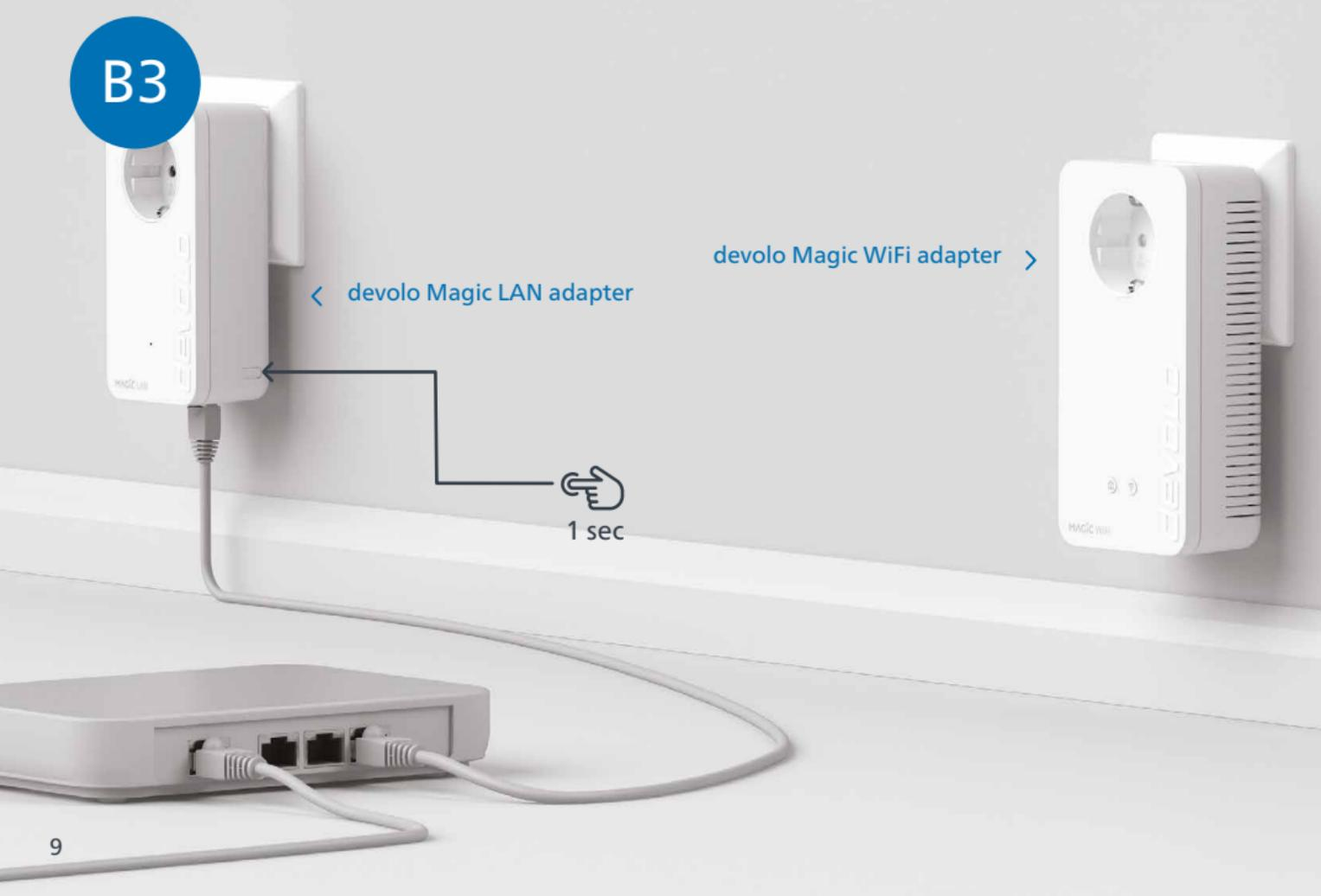
**| EN |** Within 3 minutes, press the button on the side of your devolo Magic LAN adapter which is connected to the router.
