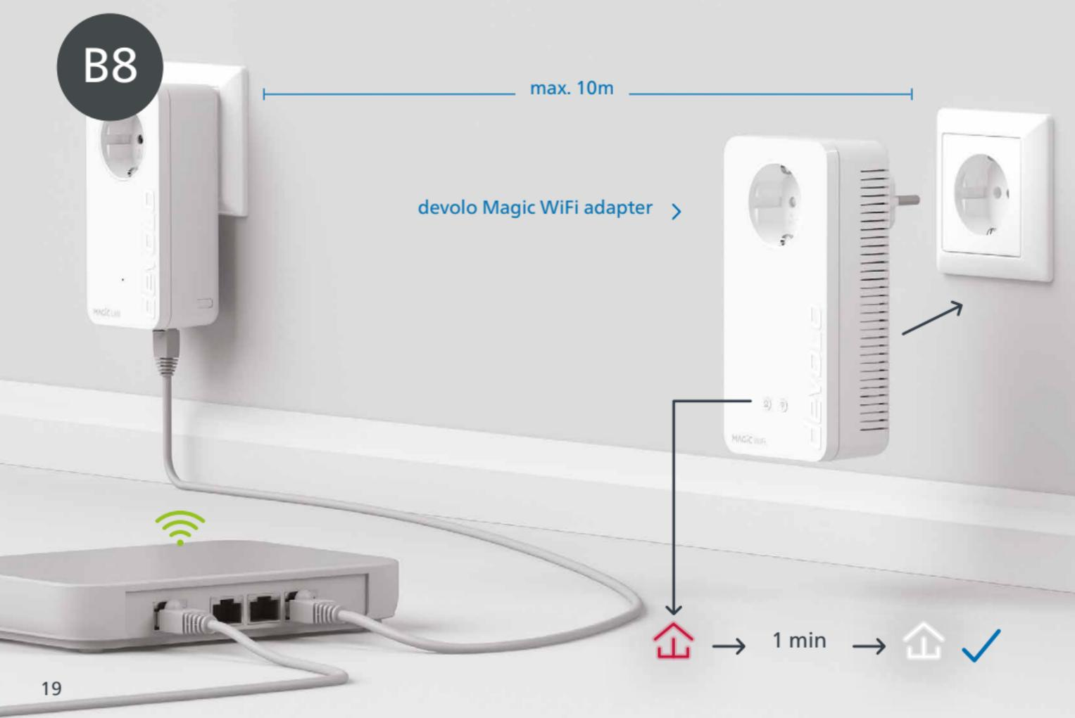
**| EN** | Connect the devolo Magic WiFi adapter for the transmission of the Wi-Fi access data to a free wall socket near your router (max. distance 10 metres) and wait around 1 minute until the LED lights up white.
