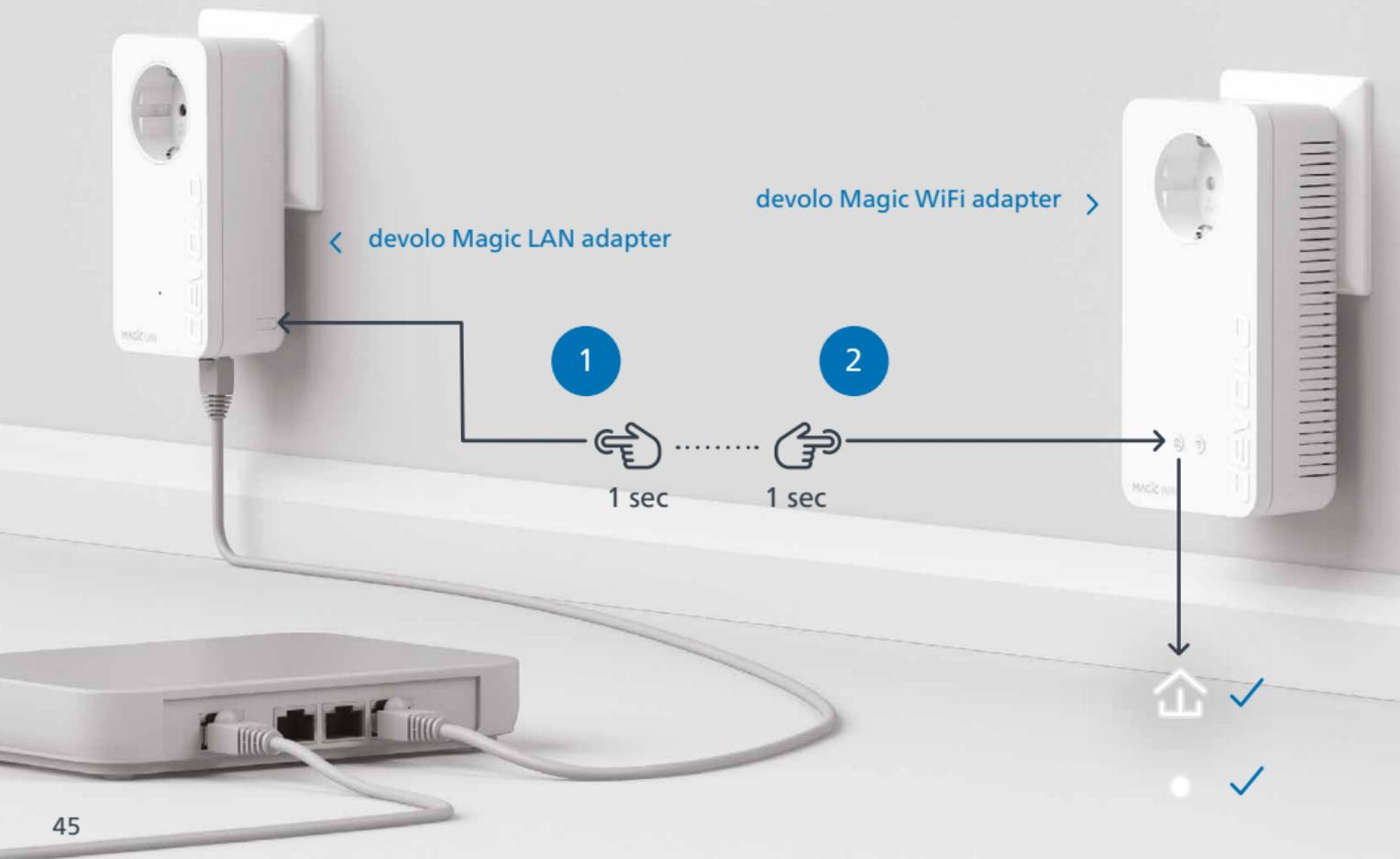
**| EN |** Within 3 minutes, press the button on the side of your devolo Magic LAN adapter which is connected to the router. Second, press the
