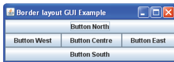
Figure 3.5 The BorderLayout manager
