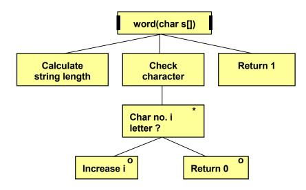
The function begins by calculating the string length. The loop 'Check character' goes through character by character and checks if it is in the interval a-z or A-Z. If so, we increase the loop counter i by 1. Otherwise we return the value 0 and the function is terminated. If all characters are letters, the loop will complete and we return 1.
