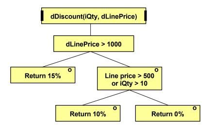
The function dDiscount() takes the quantity and line price as parameters. If the line price exceeds 1000, the discount 15 % is returned. Otherwise (i.e. the line price is less than or equal to 1000), we check if the line price exceeds 500 or the quantity exceeds 10. Then 10 % is returned. In other cases there will be no discount and 0 % is returned.
