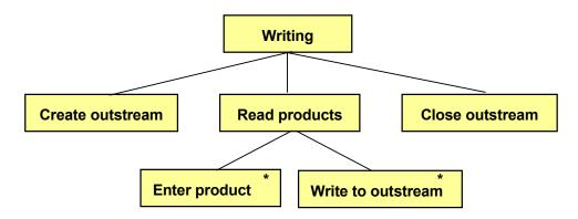
First we declare an outstream and attach it the file prodfile.txt. Entry of product names from the keyboard is made in a loop. As soon as a product name has been entered by the user, it is written to the outstream. At entry completion, we close the outstream.
