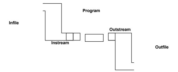
When data is to be read from a disk file (infile) to a program, it goes via an intermediary store (instream) which works as a buffer between the hard disk and the program, where data is queued to be read to the program.
