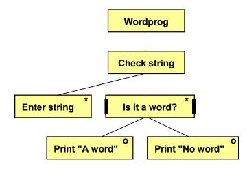
The program has a loop 'Check string'. For each turn of the loop we read a string from the keyboard. The string is sent to the function word(). If 1 is returned by the function, we print 'A word'. If 0 is returned, we print 'No word'.
